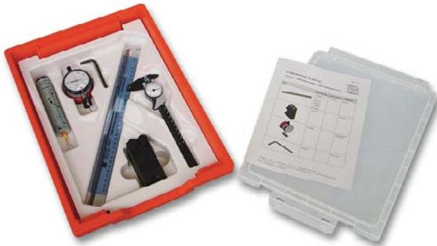
Students set up a beam on the supports and add weights to deflect the beams. An accurate dial indicator measures the deflection at the point of loading.
