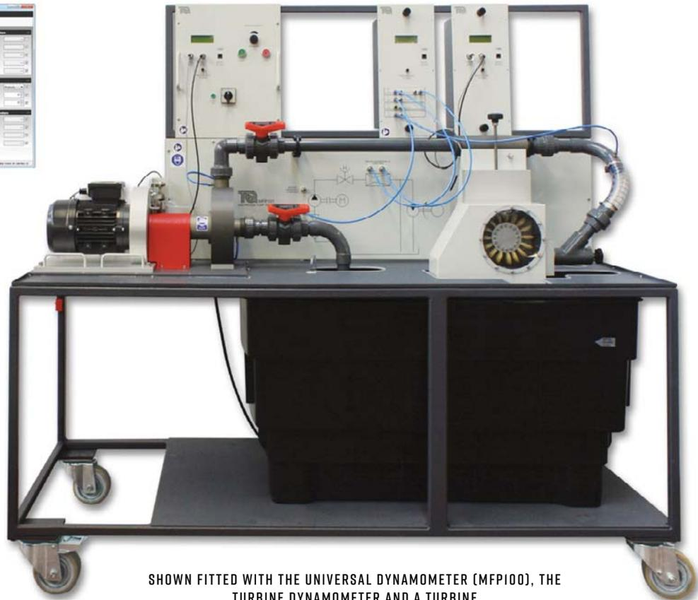
SHOWN FITTED WITH THE UNIVERSAL DYNAMOMETER (MFP100), THE TURBINE DYNAMOMETER AND A TURBINE
